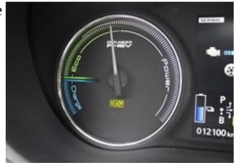
b) If gauge at full throttle (but not kick-down) points to green area, but not at the end of it, this means that **power limitation is too high** and it can be increased to improve car dynamics. Open the box and turn the internal rotary programmer one value down (this will increase the power limit with a step of 3 kW). Usually the box is set to program 2 as a factory setting, so you can switch to program 1 (program 0 = factory car).
