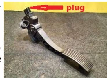
3. Unplug factory plug, by pressing lock on the plug and lifting it up. To understand how it is locked, see box wiring – it uses exactly same plug.
