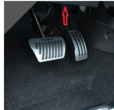
2. Find plug at accelerator pedal. Plug is at the top of pedal assembly – it can be reach easily by hand.
